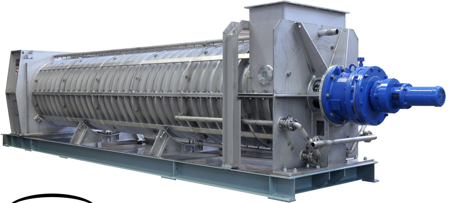
Model BHX-1000 x 5500L Screw Press (with covers removed)
